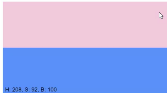
Figure 2.6.1: The finished color picker: the top half previews colors while the mouse moves, the bottom half keeps the color chosen with the last click, and the corner lists its HSB values.
